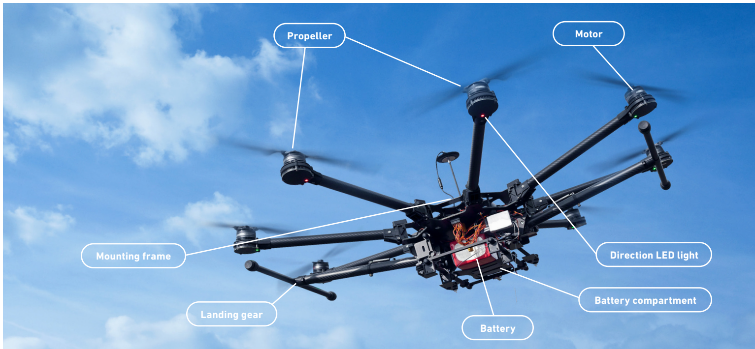
FIGURE 1—HARDWARE COMPONENTS OF A STANDARD UAV
