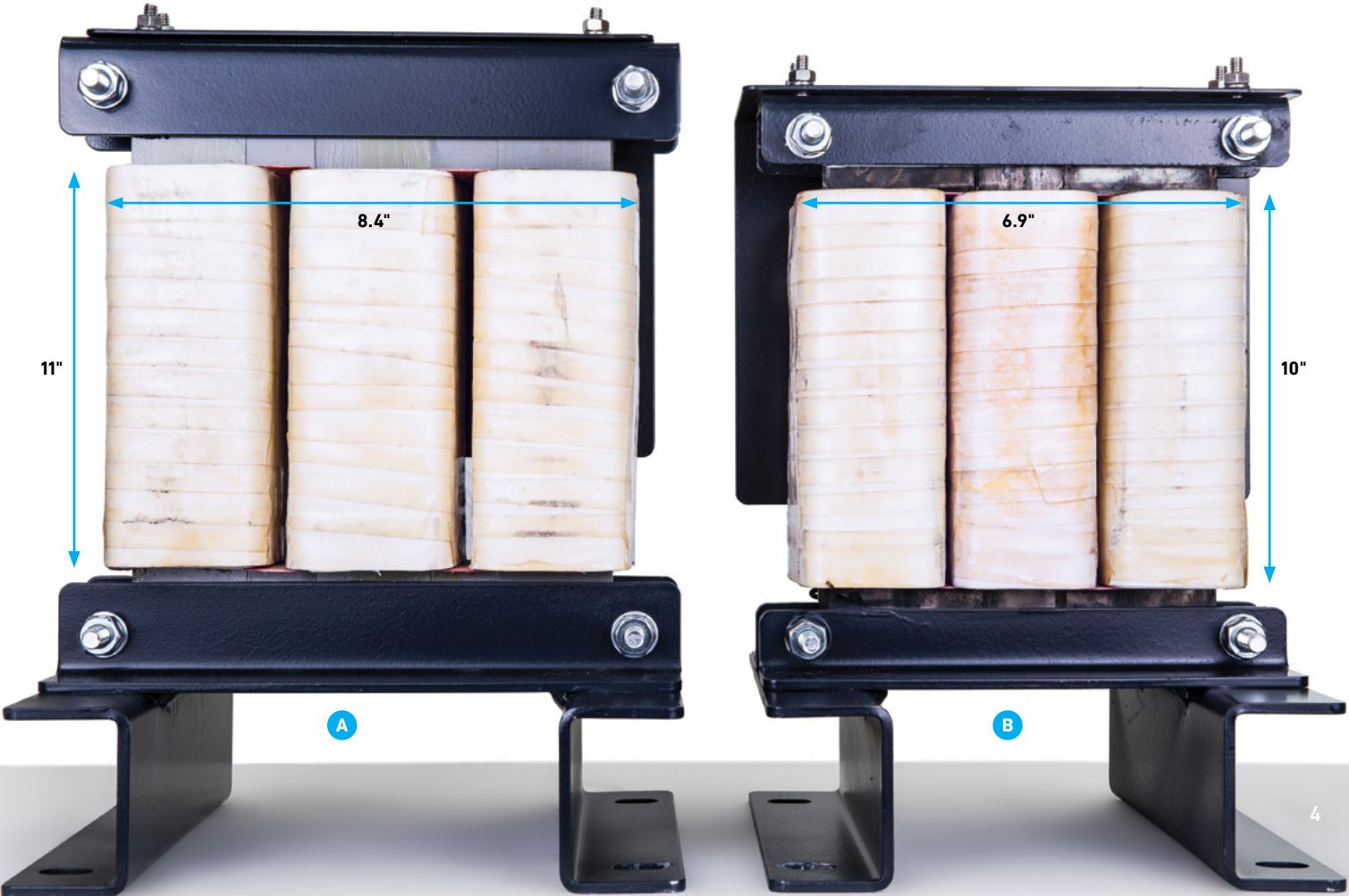
FIGURE 1 — TRANSFORMER PROTOTYPES MADE FROM GOES M6 CORE (LEFT) AND HIPERCO 50A CORE (RIGHT). THE HIPERCO 50A CORE IS 31% SMALLER AND LIGHTER.
